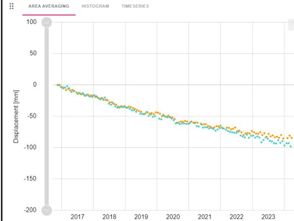
The displacement rate on this road section is higher than neighboring areas, reaching up to velocities of  $\sim -12.5$  mm/y, as compared to the rest of the road, which is around  $-3.7$  mm/y.
