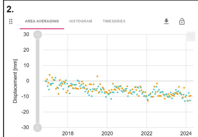
**Description:** We observe different displacement magnitudes within the same location. Time series show that the barn (1), exhibits more than twice as much displacement (up to ~5 mm/yr) as the terrain next to it (up to ~2 mm/yr). The reason for this can be local variations in soil properties and compaction occurring due to the additional load of the barn.
