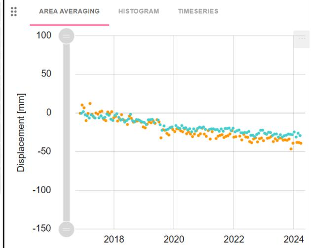
The displacement can be very localized and can correlate with local soil type. The displacement rates can be between  $\sim -2.5$  and  $-6$  mm/y
